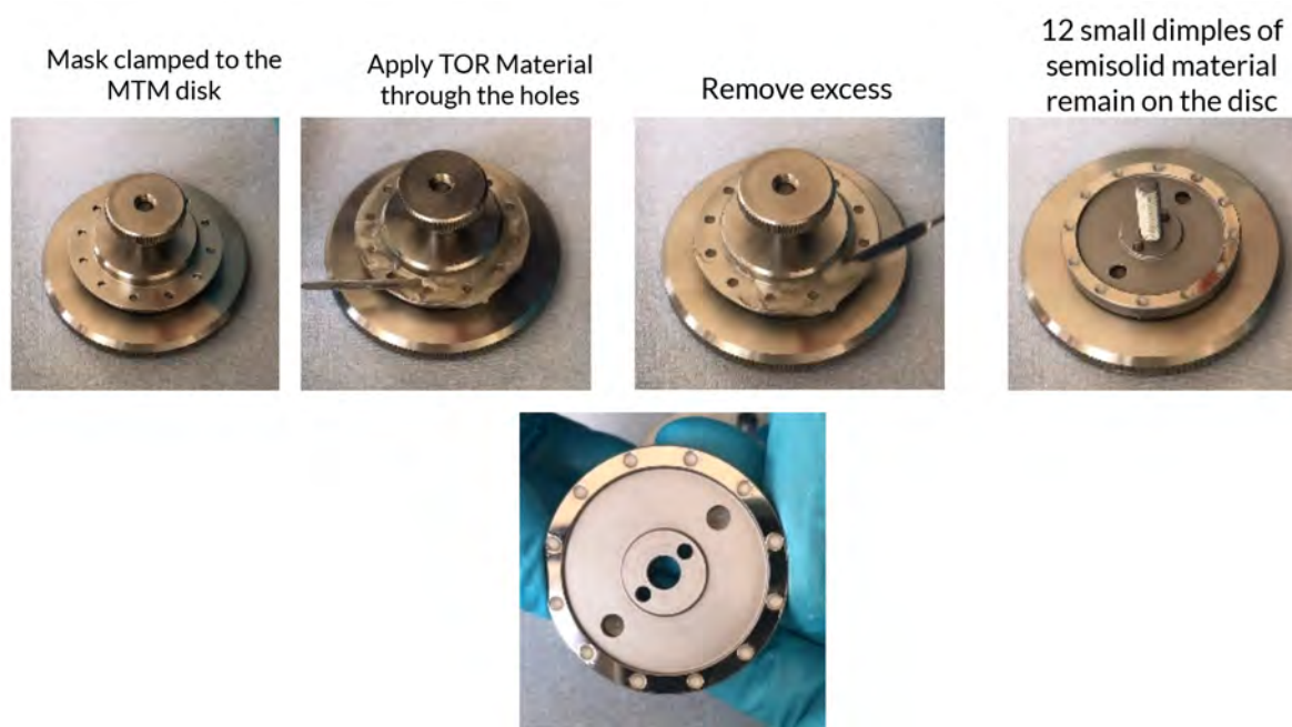
Figure 4: Photographs showing the step-by-step application of semisolid product onto the surface of a MTM disk.
